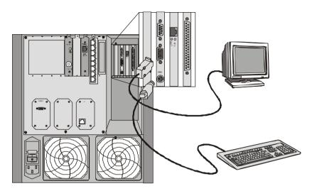
Figure 3-4: Attaching the Monitor and Key Board to the MGC-50
